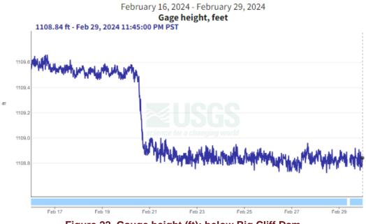
Figure 22. Gauge height (ft); below Big Cliff Dam.
