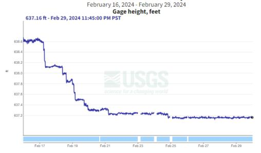
Figure 67. Gauge Height (feet); below Dexter Dam, Middle Fork Willamette.
