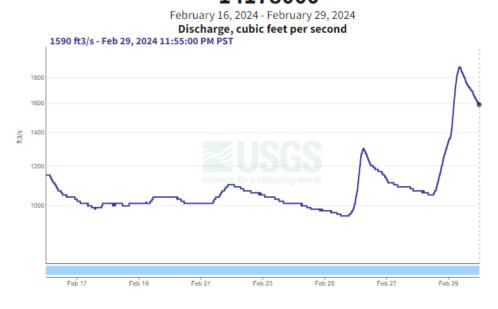
Figure 28. Discharge (cfs); Detroit Head of Reservoir – North Santiam River.
